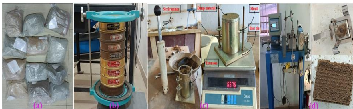
Figure 4: Collection of dump samples and geotechnical tests conducted a. collection of samples b. Sieve size analysis c. Proctor compaction d. Direct shear test.
